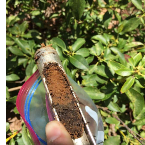
10-cm deep soil sample from a forest plots. Orange coloration indicates the presence of the iron sulfides.
