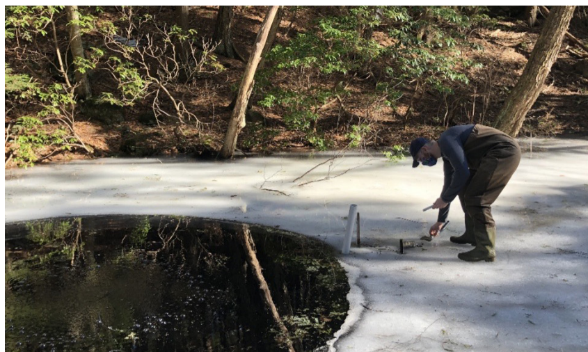
Logan places a temperature logger in one of the wood frog breeding ponds. These loggers are installed each spring, sometimes requiring breaking through the ice. Photo courtesy of Logan Billet
